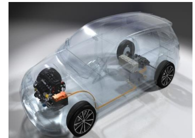
Electric Rear Drive Unit
