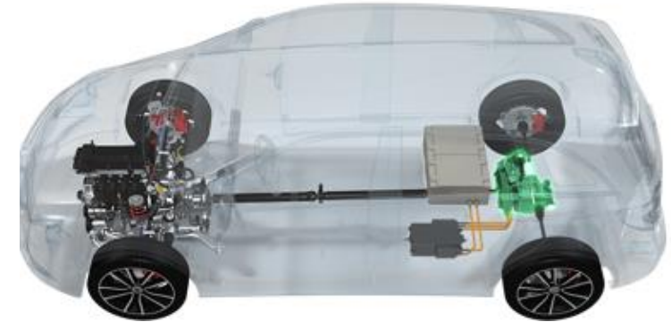
AAM P3 Rear e-Drive unit (Hybrid) Launching in 2020
