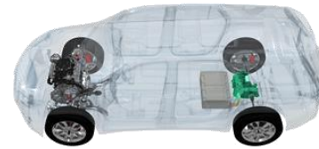
P4 SPLIT AXLE HYBRID ARCHITECTURE
